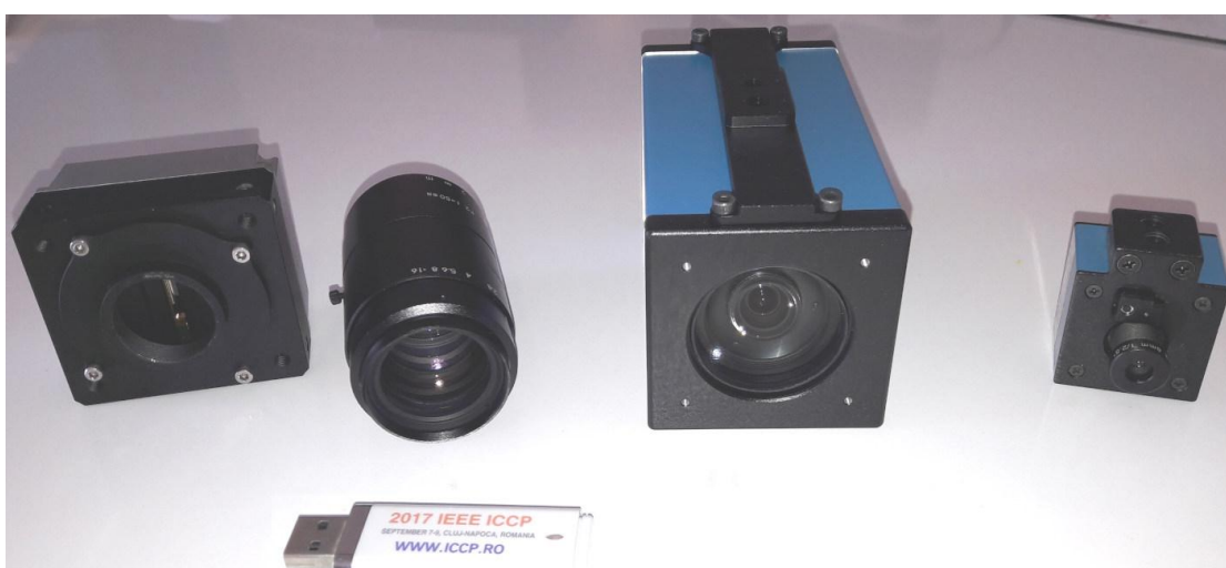
Figure 1.1. Three Industrial Machine Vision Cameras and a lens. From left to right: A CMOS line-scan Camera, its lens, a zoom controllable area-scan camera with integrated optics and a USB high-resolution auto-focus camera.
