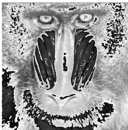
Figure 2.15. Grayscale “Mandrill” image after being low-pass filtered with wrong coefficients. The dark areas are due to the overflow of unsigned char.
