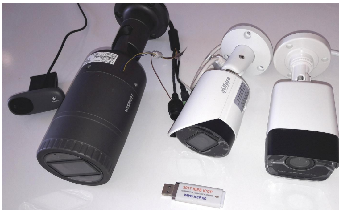
Figure 1.3. Three security cameras and a webcam. From left to right: A Logitech USB webcam, a Wisenet, a Dahua and a HikVision outdoor security cameras.
