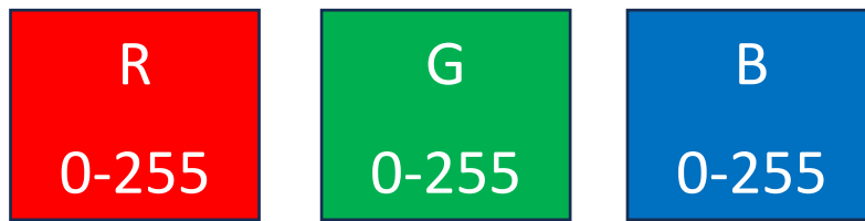
Figure 3.3. Three bytes are required to set (select) the color of a pixel.
